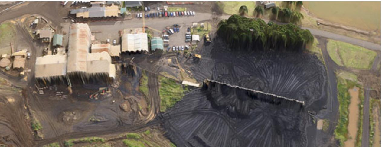
New Zealand Steel has been utilising Synergy Positioning Systems' Unmanned Aerial Vehicle (UAV) mapping technology to accurately measure stockpile volumes on a monthly basis at both its Taharoa and Waikato North Head mine sites....
