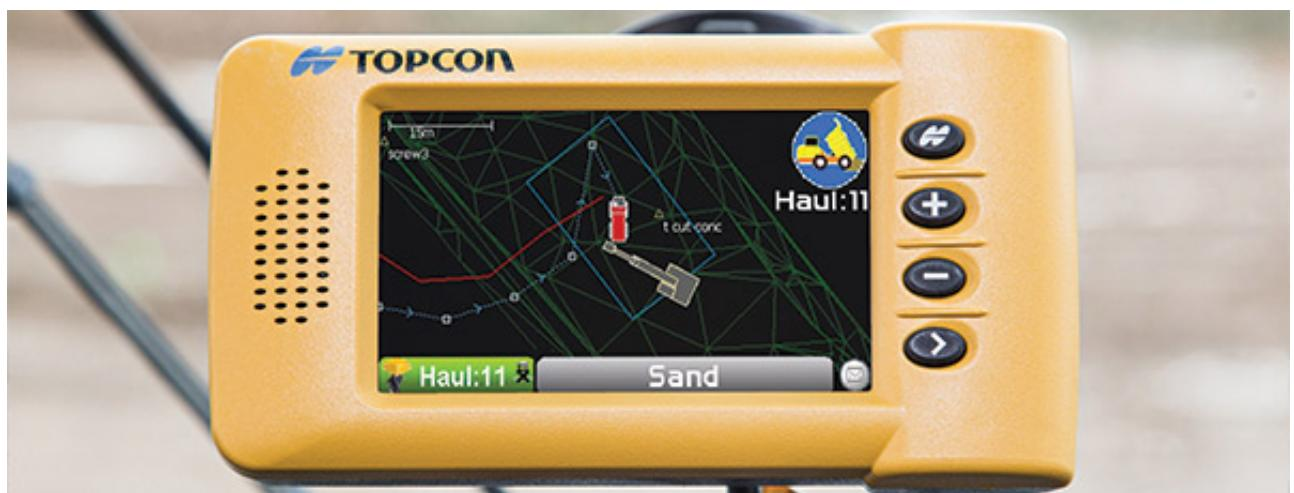
Working seamlessly within the Sitelink3D system – Topcon's unrivaled site management, data control and systems support technology – the new HT-30 module features a small, portable GPS/GPRS-enabled control box that sits inside the truck cab.
