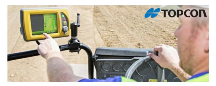
Specifically engineered for compactors, the new Topcon C-63 indicate system is designed to precisely track compaction with minimal equipment operation.
