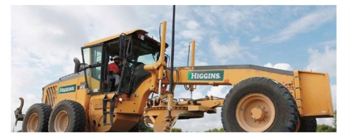
At Ngaruawahia a positive mix of operator talent and Topcon's precision 3D Machine Control technology has resulted in the successful completion of a large-scale infrastructure project, as civil contracting firm Higgins Group complete the build of a lengthy section of Waikato Expressway...
