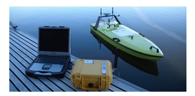
**Simplicity of Operation.** A survey tool not a science project; simply turn on the vehicle and the on-board CEESCOPE™ and start surveying. With echo sounding, positioning, data management, user control interface, RTK and data telemetry in a single enclosure there is no simpler USV to use. Minimize downtime, mobilization, and field crew headaches.
