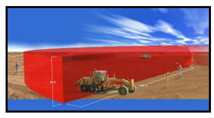
working area to 133' or 7880' horizontally. The rovers dynamically move from one transmitter to the next seamlessly.
