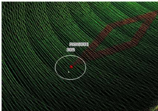
Example of measurement of GCP (measurement of apex of rhombus mark)
