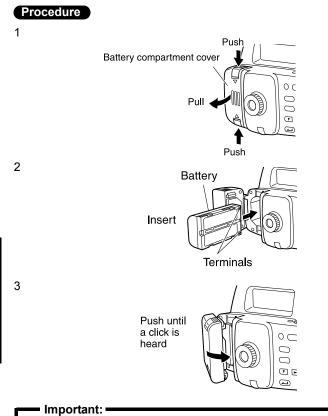
• Always turn off the power before removing the battery from the instrument. If the battery is removed when the power is still on, stored data may be lost.
