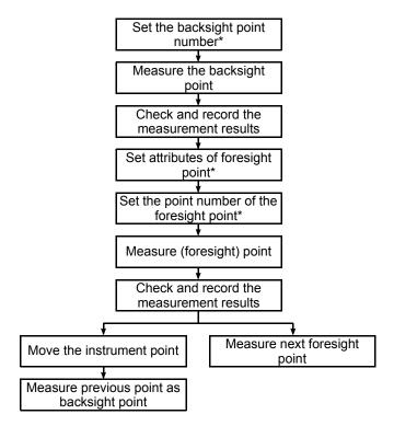
The following procedure is an example of measurement in height difference measurement mode.
