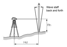
The forward and backward movement with respect to vertical position A should be equal and not in excess of 5 to 10°.
