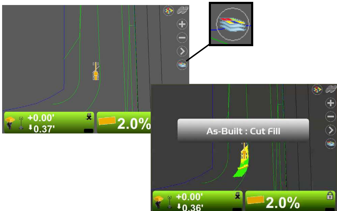
Figure 111: As-built Shortcut Button – Cut/Fill
