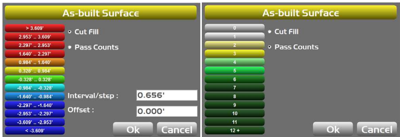
Figure 106: As-built Surface Screen
