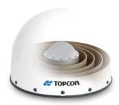
The CR-G5-C is a choke ring antenna with cavity filter based on Topcon's TA-5 full spectrum GNSS antenna element. The TA-5 antenna element utilizes an array of vertical convex dipoles. This antenna provides Full Wave tracking technology for existing and future GNSS signals.
