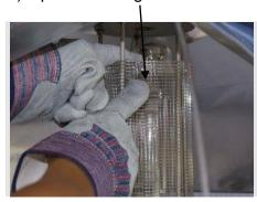
4) Insert new bulb by placing it in the lower socket first. Then gently press down bulb and place in upper socket. Make sure it sits correct and firm.
