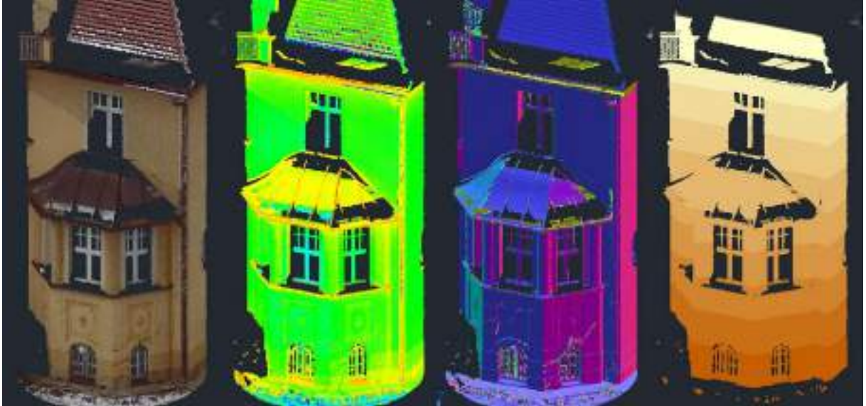
Figure 2 Visualisation styles (from left to right): RGB real colours, intensity (spectral colours), normal appearance, elevation slices
