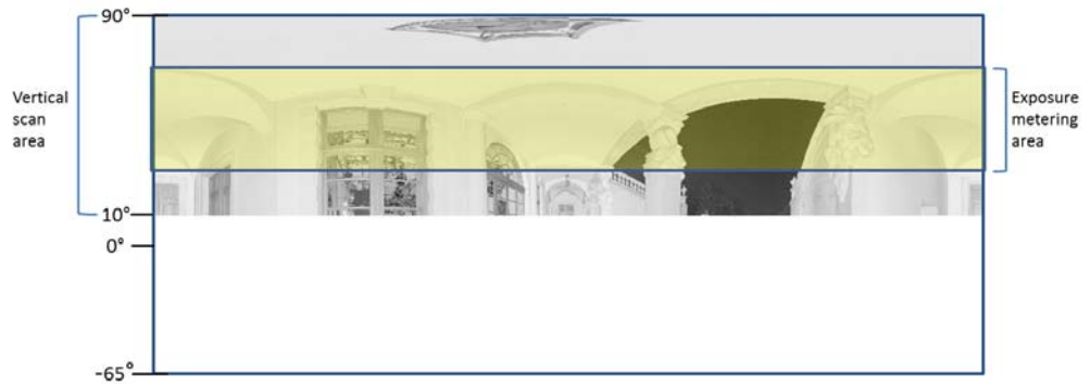
Figure 7-46: Exposure metering area for a limited vertical scan area set to e.g. 10° to 90°
