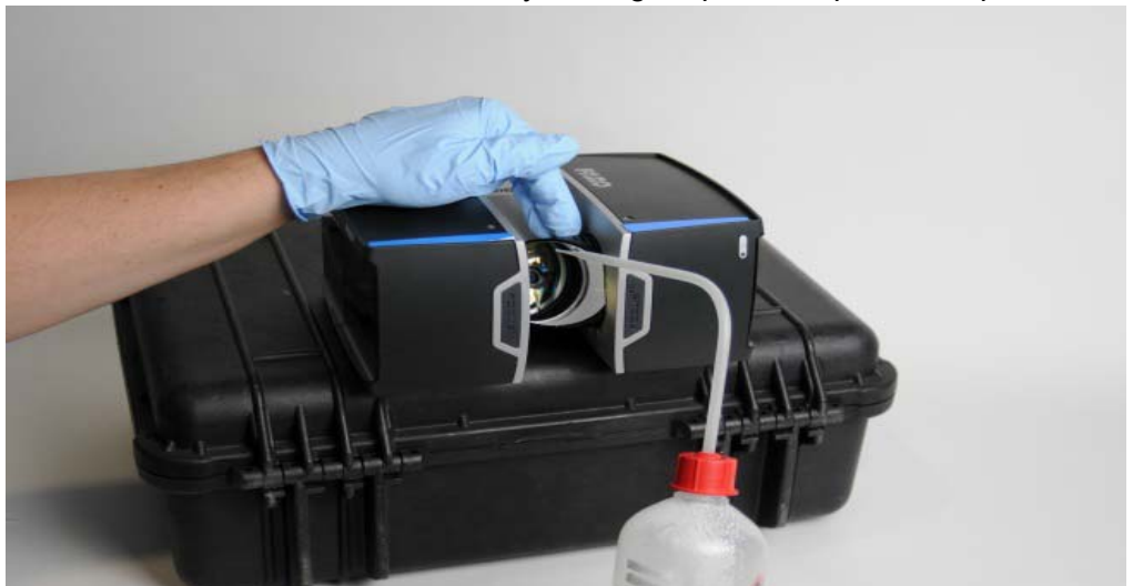
Figure 9-111: Cleaning mirror module or sensor cover
