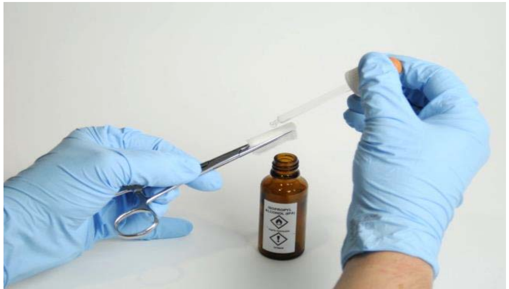
Figure 9-105: Soaking the cleaning pad
