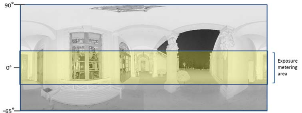
Figure 6-28: Exposure metering area (highlighted yellow) for the full vertical scan area
