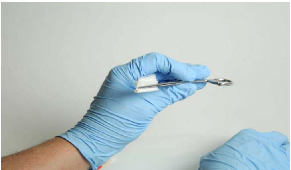
Figure 9-104: Creating a T-shaped cleaning pad (2)
