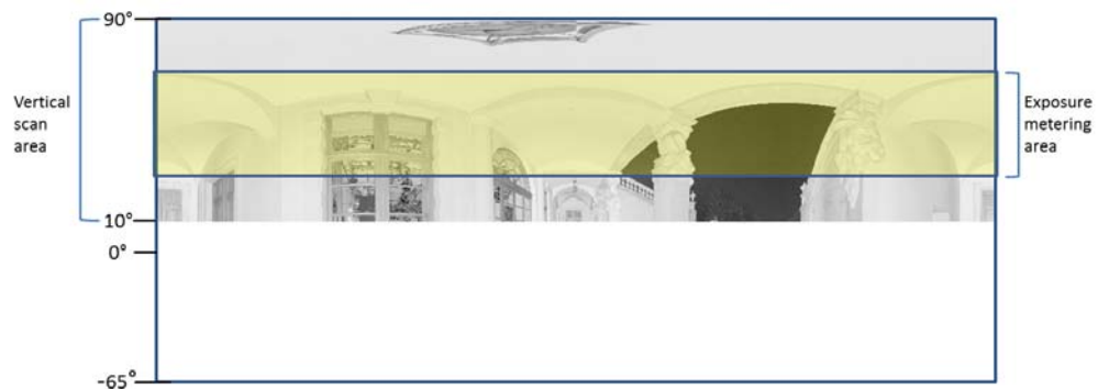
Figure 6-29: Exposure metering area for a limited vertical scan area set to e.g. 10^\circ to 90^\circ
