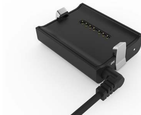
Figure 6-11: Power Dock battery charger with connected power cable
