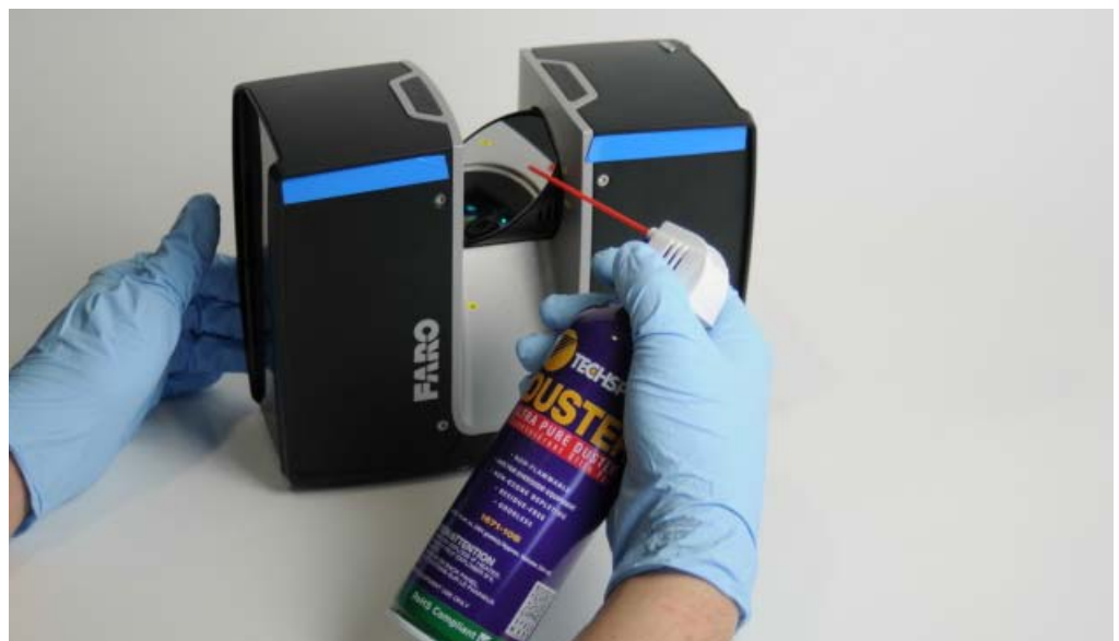
Figure 9-108: Dry pre-cleaning by compressed air or duster cleaning spray
