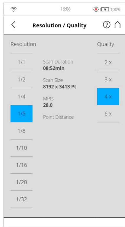
Figure 7-40: Scan Parameters, Resolution, and Quality
