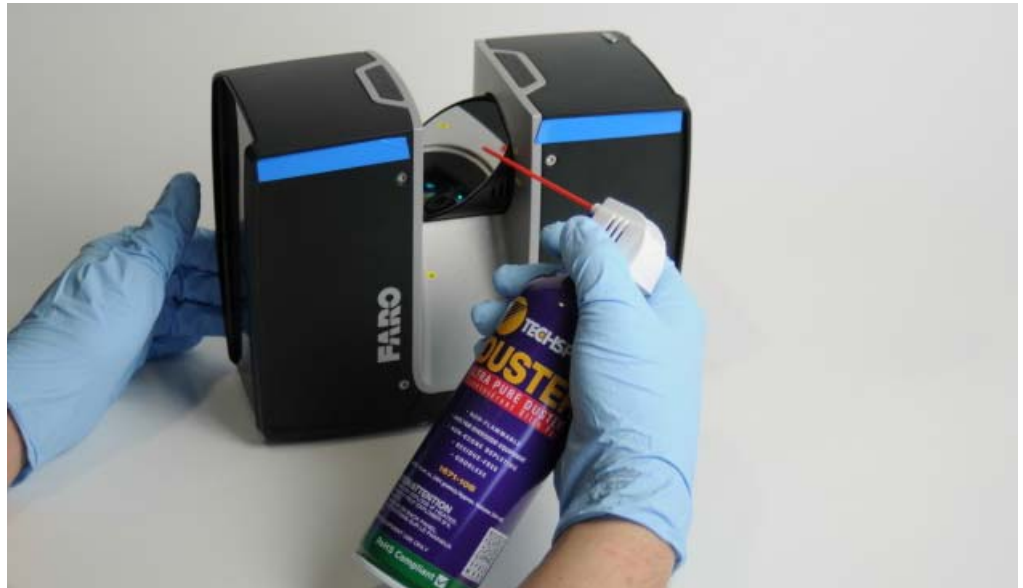
Figure 9-98: Dry pre-cleaning with compressed air or duster cleaning spray
