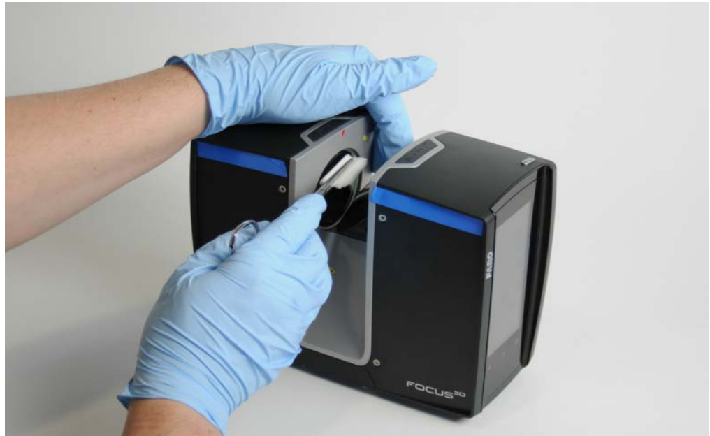
Figure 9-107: Cleaning sensor cover with pad and isopropyl alcohol or cleaning fluid
