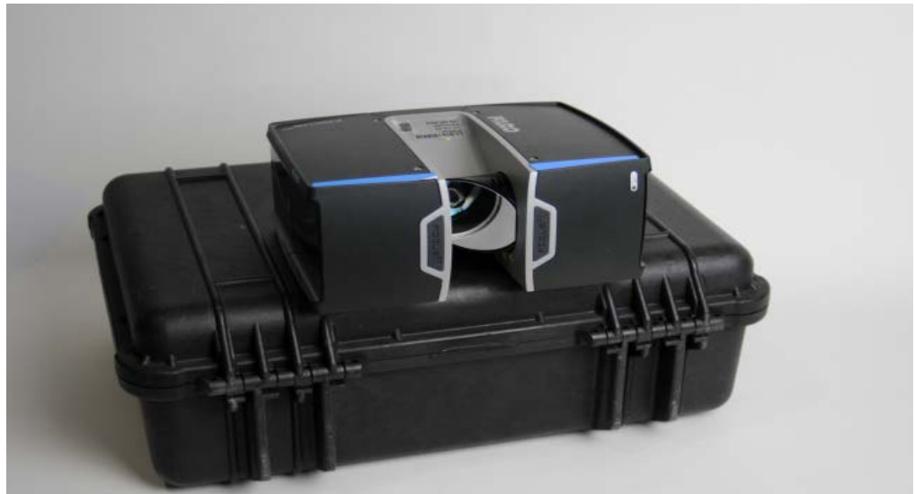
Figure 9-109: Transport box with laser scanner turned and laid on top, with the mirror module facing outwards
