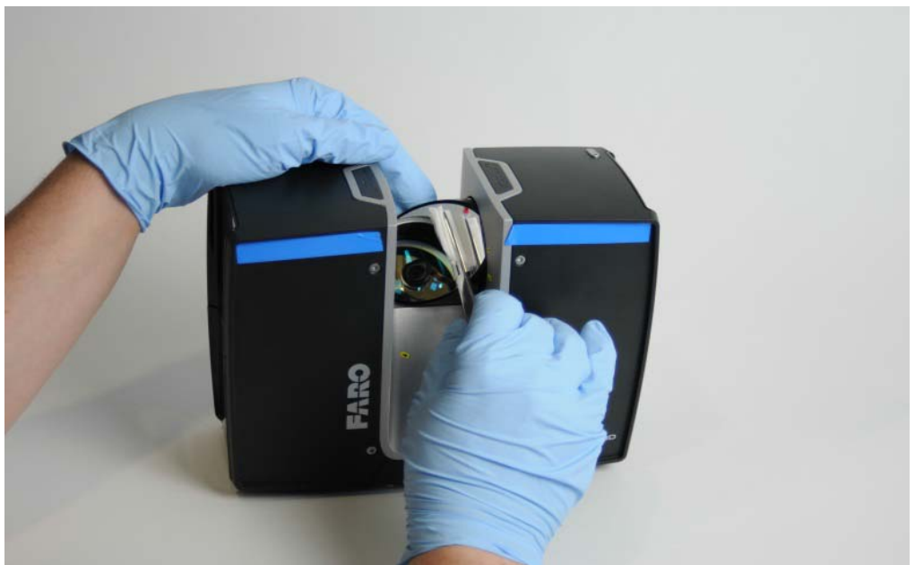
Figure 9-106: Cleaning mirror module with pad and isopropyl alcohol or cleaning fluid
