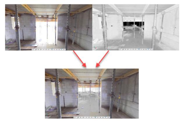
The laser light does not provide color information, so areas illuminated only by the laser are grayscale.
